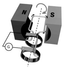
The plane of the loop is parallel to the external magnetic field so the induced current is at a maximum.
