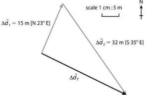
This figure shows the given vectors, with the tip of  $\Delta \vec{d}_1$  joined to the tail of  $\Delta \vec{d}_2$ . The resultant vector  $\Delta \vec{d}_T$  is drawn in black from the tail of  $\Delta \vec{d}_1$  to the tip of  $\Delta \vec{d}_2$ . Using a compass, the direction of  $\Delta \vec{d}_T$  is [E 27° S].  $\Delta \vec{d}_T$  measures 5.4 cm in length, so using the scale of 1 cm : 5 m, the actual magnitude of  $\Delta \vec{d}_T$  is 27 m.
