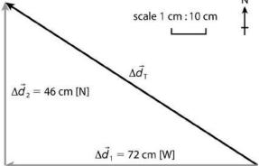
This figure shows the given vectors, with the tip of  $\Delta \vec{d}_1$  joined to the tail of  $\Delta \vec{d}_2$ . The resultant vector  $\Delta \vec{d}_T$  is drawn in black from the tail of  $\Delta \vec{d}_1$  to the tip of  $\Delta \vec{d}_2$ . Using a compass, the direction of  $\Delta \vec{d}_T$  is [W 33° N].  $\Delta \vec{d}_T$  measures 8.5 cm in length, so using the scale of 1 cm : 10 cm, the actual magnitude of  $\Delta \vec{d}_T$  is 85 cm.
