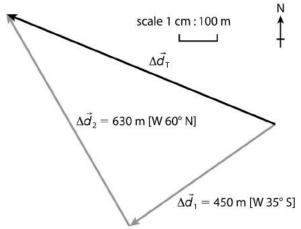
This figure shows the given vectors, with the tip of  $\Delta \vec{d}_1$  joined to the tail of  $\Delta \vec{d}_2$ . The resultant vector  $\Delta \vec{d}_T$  is drawn in black from the tail of  $\Delta \vec{d}_1$  to the tip of  $\Delta \vec{d}_2$ . Using a compass, the direction of  $\Delta \vec{d}_T$  is [W 23° N].  $\Delta \vec{d}_T$  measures 7.4 cm in length, so using the scale of 1 cm : 100 m, the actual magnitude of  $\Delta \vec{d}_T$  is 740 m.
