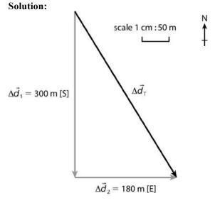
This figure shows the given vectors, with the tip of  $\Delta \vec{d}_1$  joined to the tail of  $\Delta \vec{d}_2$ . The resultant vector  $\Delta \vec{d}_1$  is drawn in black from the tail of  $\Delta \vec{d}_1$  to the tip of  $\Delta \vec{d}_2$ . Using a compass, the direction of  $\Delta \vec{d}_T$  is [S 31° E].  $\Delta \vec{d}_T$  measures 7.0 cm in length, so using the scale of 1 cm : 50 m, the actual magnitude of  $\Delta \vec{d}_T$  is 350 m.
