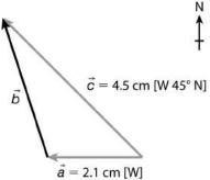
This figure shows the given vectors, with the tail of  $\vec{a}$  joined to the tail of  $\vec{c}$ . The missing vector  $\vec{b}$ is drawn in black from the tip of  $\vec{a}$  to the tip of  $\vec{c}$ . Using a compass, the direction of  $\vec{b}$  is [W 74° N].  $\vec{b}$  measures 3.4 cm in length. **Statement:** Vector  $\vec{b}$  is 3.4 m [W 74° N]. **Note:** Figure 5 in the Student Book was modified after the first printing. The solutions below reflect this change.
