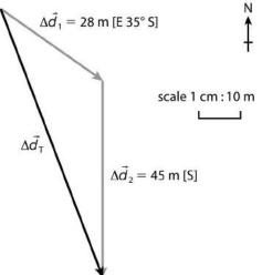
This figure shows the given vectors, with the tip of  $\Delta \vec{d}_1$  joined to the tail of  $\Delta \vec{d}_2$ . The resultant vector  $\Delta \vec{d}_T$  is drawn in black from the tail of  $\Delta \vec{d}_1$  to the tip of  $\Delta \vec{d}_2$ . Using a compass, the direction of  $\Delta \vec{d}_T$
