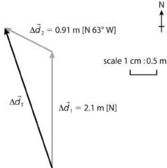
This figure shows the given vectors, with the tip of  $\Delta \vec{d}_1$  joined to the tail of  $\Delta \vec{d}_2$ . The resultant vector  $\Delta \vec{d}_{T}$  is drawn in black from the tail of  $\Delta \vec{d}_{T}$  to the tip of  $\Delta \vec{d}_2$ . Using a compass, the direction of  $\Delta \vec{d}_T$ is [N 18° E].  $\Delta \vec{d}_{T}$  measures 5.2 cm in length, so using the scale of 1 cm : 0.5 m, the actual magnitude of  $\Delta \vec{d}_{\rm T}$  is 2.6 m.
