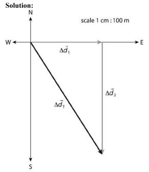
This figure shows the given vectors, with the tip of  $\Delta \vec{d}_1$  joined to the tail of  $\Delta \vec{d}_2$ . The resultant vector  $\Delta \vec{d}_1$  is drawn in black from the tail of  $\Delta \vec{d}_1$  to the tip of  $\Delta \vec{d}_2$ . Using a compass, the direction of  $\Delta \vec{d}_T$  is [E 58° S].  $\Delta \vec{d}_T$  measures 6.7 cm in length, so using the scale of 1 cm : 100 m, the actual magnitude of  $\Delta \vec{d}_T$  is 670 m.
