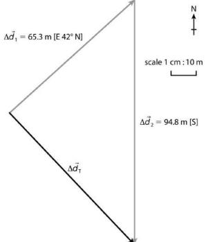
This figure shows the given vectors, with the tip of  $\Delta \vec{d}_1$  joined to the tail of  $\Delta \vec{d}_2$ . The resultant vector  $\Delta \vec{d}_1$  is drawn in black from the tail of  $\Delta \vec{d}_1$  to the tip of  $\Delta \vec{d}_2$ . Using a compass, the direction of  $\Delta \vec{d}_1$  is [W 46° S].  $\Delta \vec{d}_1$  measures 7.05 cm in length, so using the scale of 1 cm : 10 m, the actual magnitude of  $\Delta \vec{d}_1$  is 70.5 m.
