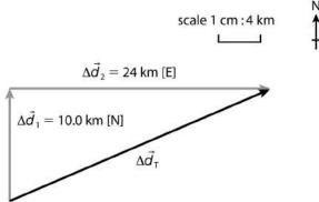
This figure shows the given vectors, with the tip of  $\Delta \vec{d}_1$  joined to the tail of  $\Delta \vec{d}_2$ . The resultant vector  $\Delta \vec{d}_T$  is drawn in black from the tail of  $\Delta \vec{d}_1$  to the tip of  $\Delta \vec{d}_2$ . Using a compass, the direction of  $\Delta \vec{d}_T$  is [N 67° E].  $\Delta \vec{d}_T$  measures 6.5 cm in length, so using the scale of 1 cm : 4 km, the actual magnitude of  $\Delta \vec{d}_T$  is 26 km.
